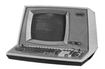
MODEL 2226 CRT/KEYBOARD CONSOLE The Model 2226 Integrated Upper/Lowercase Alphanumeric/BASIC Keyboard has two modes of operation: Keyword/A and A/a. The mode is selected by the toggle switch in the upper left-hand corner of the keyboard. In Keyword/A mode, shifted alpha keys produce BASIC words; unshifted alpha keys produce uppercase letters. A/a mode functions as a standard typewriter. Unshifted alpha keys produce lowercase letters; shifted alpha keys produce uppercase letters.
