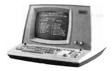
The Model '226 is comparable to the 2220 Console (see Product Bulletin No. 101). The major differences are the enlarged CRT and the removal of the Tape Drive.
