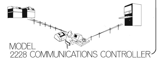
The Model 2228 Communications Controller can be plugged into an I/O slot in one of the following 2200 Series CPU models with 8K memory: the Model 2200T, the Model 2200S with Option 23 or 24, and the Model 2200B or C with Option 2 (the General I/O ROM). The System 2200 configuration must include a keyboard and a CRT since an operator uses special function keys on the keyboard to control the communications application and receives status information on the CRT
