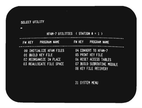
KFAM subroutines are the operational heart of the Key File Access Method. These subroutines, when incorporated into a user-written application program, can open and close KFAM files, locate random or sequential user file records, and add or delete keys in the key file. The following are important KFAM features.
