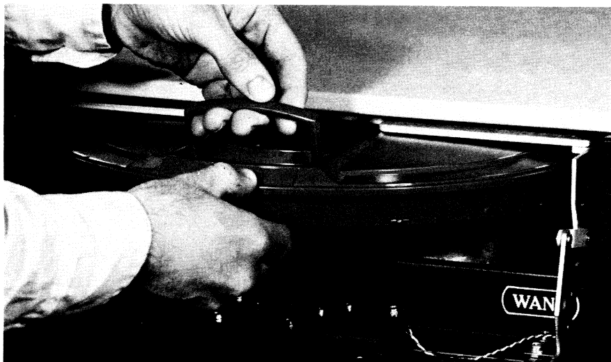
Figure 2-5. Removing the Disk Cartridge
