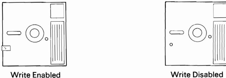
**Figure 3-1. The Write-Protect Feature on a DSDD Diskette**
