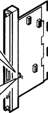
**2** If system is used as a stand-alone CPU, set jumper shorting pins 2 and 3 (BUS position).
